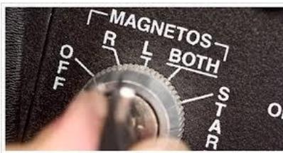
In most cases this is caused by a single spark plug which has become fouled (usually because of a too rich mixture during a too long idle period prior to takeoff). If both left and right are rough, then you should stop and cancel your flight because the following
