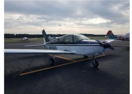
Very similar in appearance to a Cherokee except for its longer wings. This airplane features a rear storage area and a Garmin GTN 650 GPS to display all ADS-b IN data.
