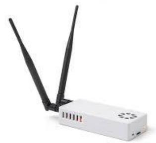
The purpose of the Stratux is to add the ability to make use of the ADS-b IN signal which is broadcast to all aircraft. If you have a tablet or an iPad which can receive Wi-Fi then all you need is an application which can display
