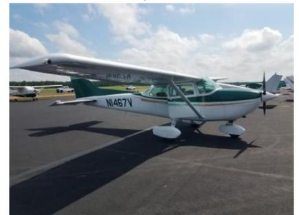
All of you are familiar with a Cessna 172 and the XP model adds an adjustable pitch propeller. Our aircraft includes a GTN 650 GPS for ADS-b IN display. This aircraft requires a brief checkout procedure before you are authorized to fly it due to the addition of the adjustable pitch propeller.
