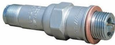
The normal scenario is this. The engine is running otherwise okay but when you run up the engine RPM and move the mag switch from left to right you notice that one side is rough while the other runs smooth.
