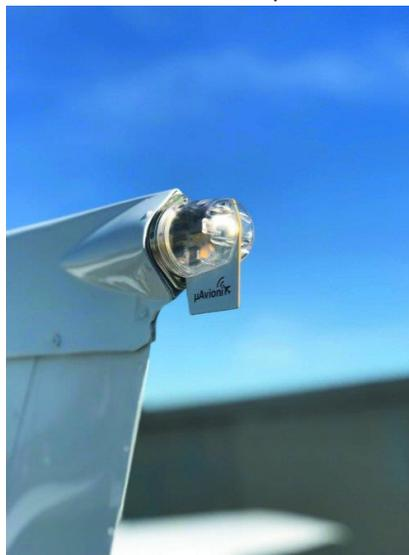
This mounts in the position of the tail nav light and provides ADS-b OUT to ATC.
