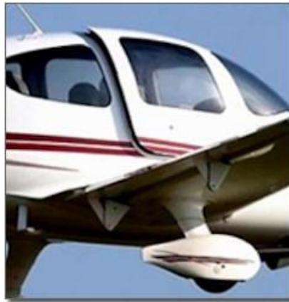
While the opening of the door is startling when it happens, you should not let it worry you. The picture above shows the maximum amount the door will open in flight. Wind pressure will hold it in this position.
