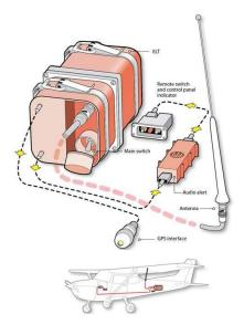
ELTs are designed to automatically activate in the event of a significant impact or crash. Modern ELTs are equipped with accelerometers or G-switches that detect sudden deceleration, such as that experienced during a crash.
